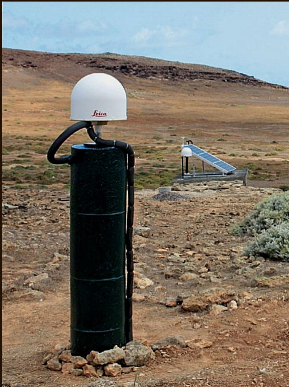
128 - In 2011 Leica Geosystems delivered a GNSS reference station to Selvagem Grande. Sensors record meteo data and send the results via satellite to the DRIGOT headquarters in Funchal, Madeira (photo: Luis Santos). The station has its own power supply through a solar/wind solution.
